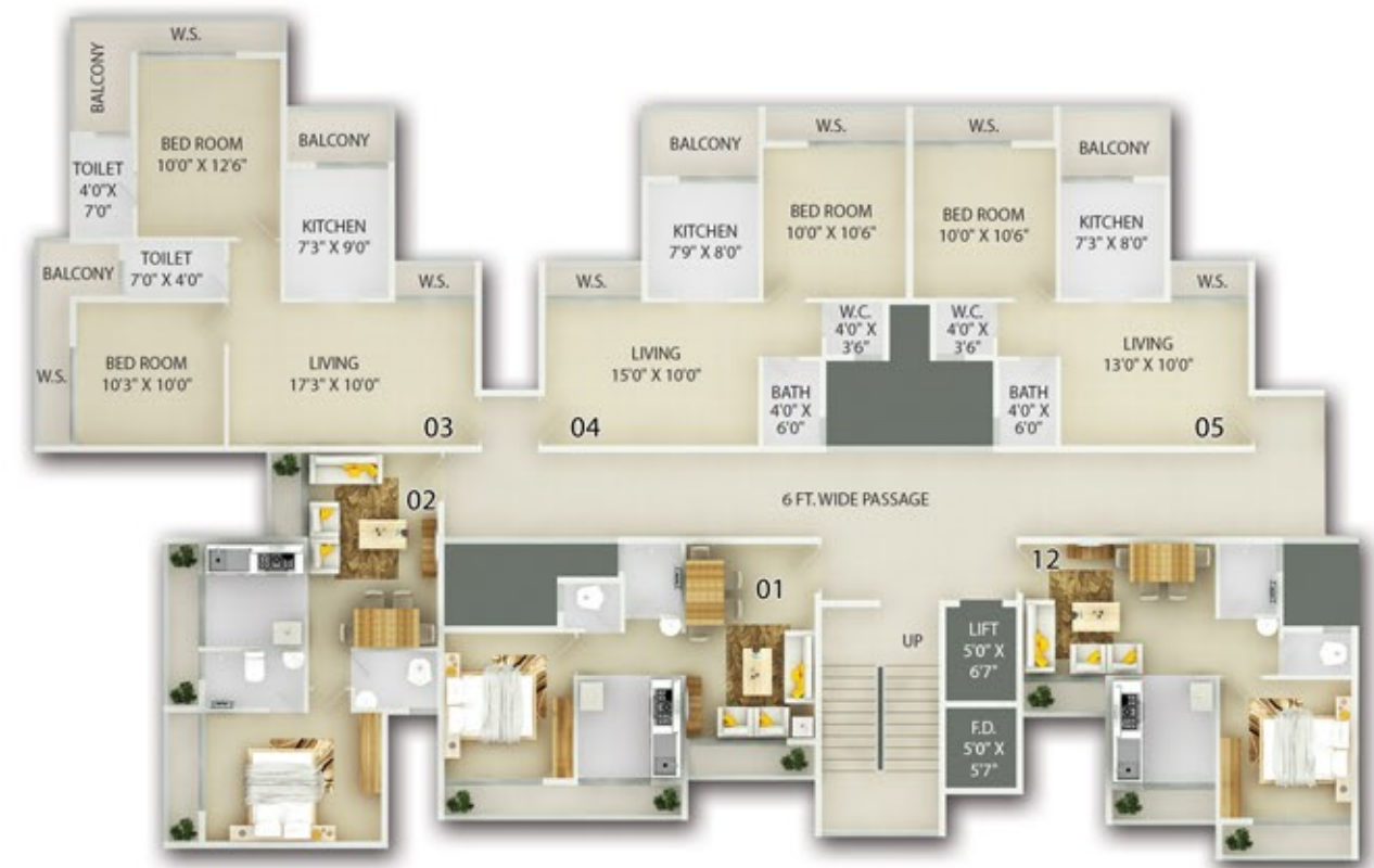
WING A | TYPICAL 3RD TO 7TH FLOOR
